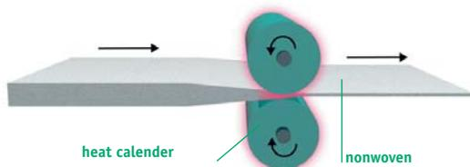
crimped staple fibres in our nonwoven products, Secutex® and Terrafix® are produced with a firm interlocking bond and exhibit high abrasion resistance. With need-
